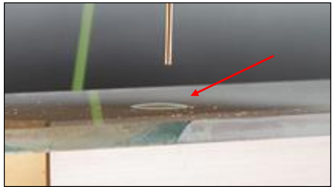
Fig CG04-02 Sheeting of Water (Low Contact Angle)
